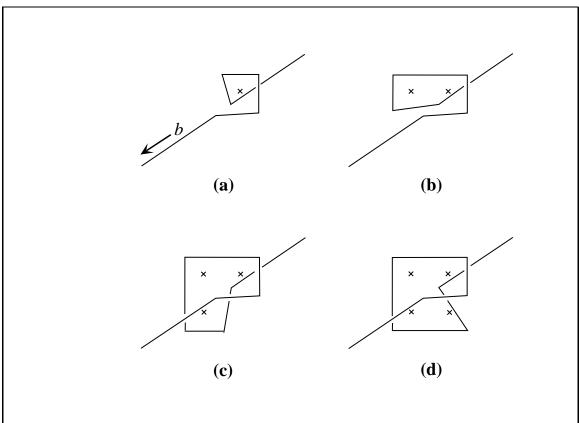
Figure 21-4: Left-hand screw dislocation in a primitive cubic crystal collects 1, 2, 3, and 4 vacancies.
