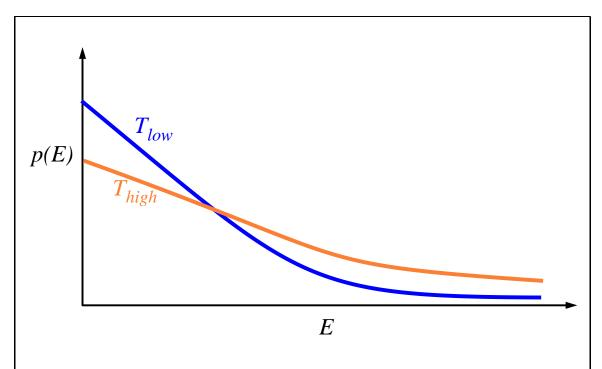
Figure 14-1: Schematic illustration of the distribution of energies at a fixed temperature, plotted for two different temperatures.  $P(E) = \exp(-E/kT)/Z$  where Z is the normalizing factor (partition function) Z, such that  $1 = \sum_E P(E)$ .
