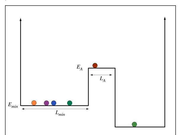
Figure 14-2: Simple model of activated process occurring between two square wells with an activation barrier of height  $E_A$ .
