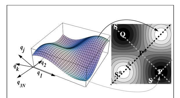
Figure 14-4: A schematic representation of the 3N-dimensional (positions) surface for a crystal with N sites. The minima are located at P and Q and it may be supposed, for simplicity, that a particle that jumps from P to Q does so along the trajectory S crossing through a maximum of width  $\delta$  at the saddle point  $A^*$  which is located at the minium along the ridge  $S^*$ .
