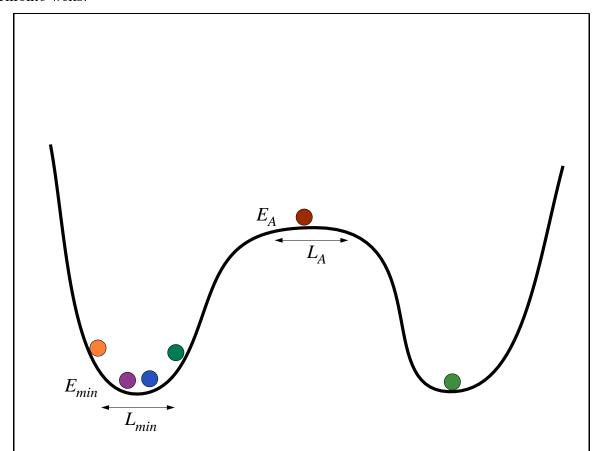
Figure 14-3: Modification to the simple square wells activated process by a harmonic potential for the equilibrium and saddle points.
