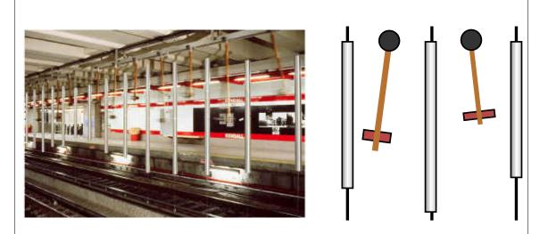
Figure 23-28: Picture and illustration of the bells at Kendall square. Many people shake the handles vigorously but with apparently no pleasant effect. The concept of resonance can be used to operate the bells efficiently Perturb the handle slightly and observe the frequencies of the the pendulums—select one and wiggle the handle at the pendulum's characteristic frequency. The amplitude of that pendulum will increase and eventually strike the neighboring tubular bells.
