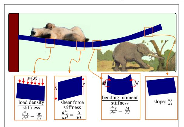
$\label{eq:Figure 21-26} Figure \ 21-26: The shape of a loaded beam is determined by the loads applied over its length and its boundary conditions. The beam curvature is related to the local moment (imagine two handles rotated in opposite directions on a free beam) divided by the effective beam stiffness. Shear forces are related to the rate of change of moment along the beam.$
