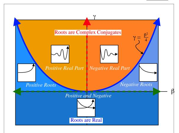
Figure 21-25: The behaviors of the linear homogeneous second-order ordinary differential equation  $\frac{d^2y}{dx^2} + \beta \frac{dy}{dx} + \gamma y = 0$  plotted according the behavior of the solutions for all  $\beta$  and  $\gamma$ .
