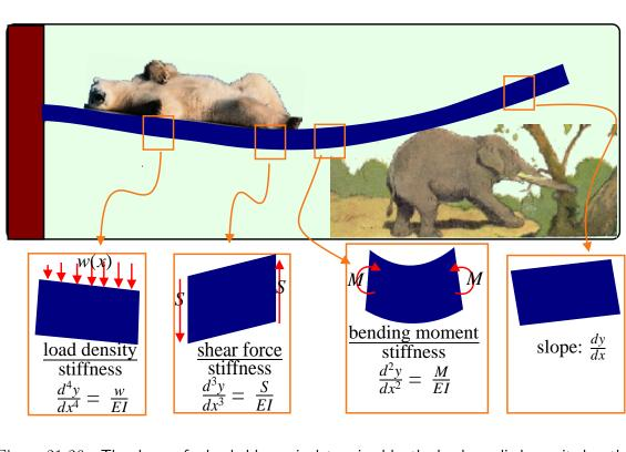
Figure 21-26: The shape of a loaded beam is determined by the loads applied over its length and its boundary conditions. The beam curvature is related to the local moment (imagine two handles rotated in opposite directions on a free beam) divided by the effective beam stiffness. Shear forces are related to the rate of change of moment along the beam. (Polar Bear Photo Art Wolfe The Zone Network http://classic.mountainzone.com/climbing/greenland/graphics/polar-bear.html )
