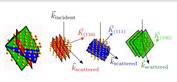
Figure 18-19: Illustration of scattering off of periodic planes and definition of scattering vector.
