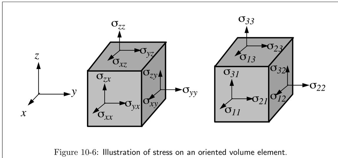
Figure 10-6: Illustration of stress on an oriented volume element.
