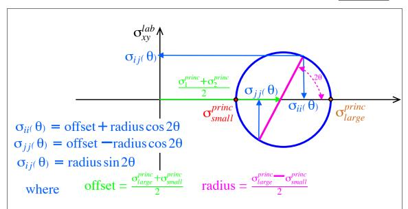
Figure 10-8: Mohr's circle of stress is a way of graphically representing the two-dimensional stresses of identical stress states, but in rotated laboratory frames.
