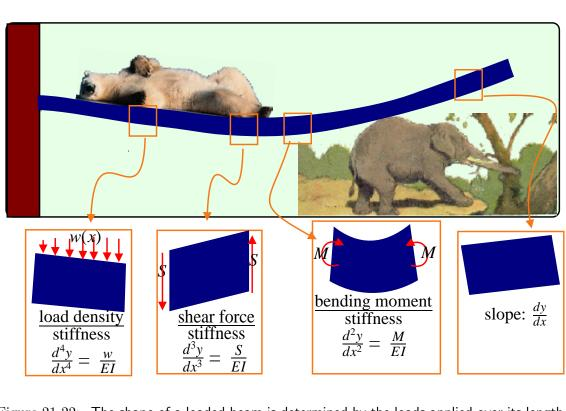
Figure 21-22: The shape of a loaded beam is determined by the loads applied over its length and its boundary conditions. The beam curvature is related to the local moment (imagine two handles rotated in opposite directions on a free beam) divided by the effective beam stiffness. Shear forces are related to the rate of change of moment along the beam. (Polar Bear Photo Art Wolfe The Zone Network http://classic.mountainzone.com/climbing/greenland/graphics/polar-bear.html )
