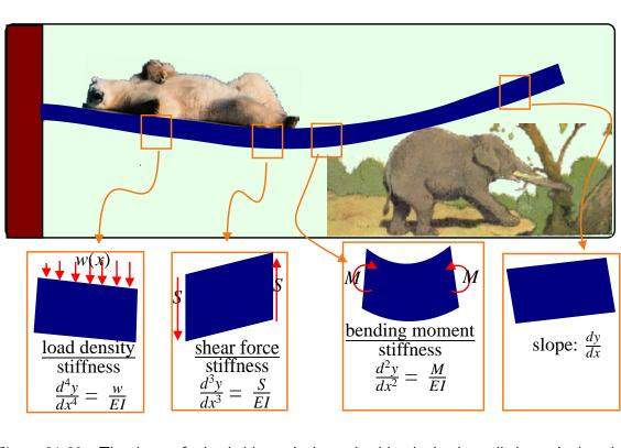
Figure 21-22: The shape of a loaded beam is determined by the loads applied over its length and its boundary conditions. The beam curvature is related to the local moment (imagine two handles rotated in opposite directions on a free beam) divided by the effective beam stiffness. Shear forces are related to the rate of change of moment along the beam. (Polar Bear Photo Art Wolfe The Zone Network http://classic.mountainzone.com/climbing/greenland/graphics/polar-bear.html )
