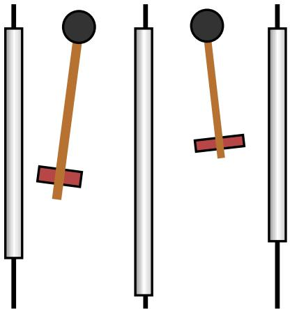
Figure 23-24: Picture and illustration of the bells at Kendall square. Many people shake the handles vigorously but with apparently no pleasant effect. The concept of resonance can be used to operate the bells efficiently. Perturb the handle slightly and observe the frequencies of the the pendulums—select one and wiggle the handle at the pendulum's characteristic frequency. The amplitude of that pendulum will increase and eventually strike the neighboring tubular bells.
