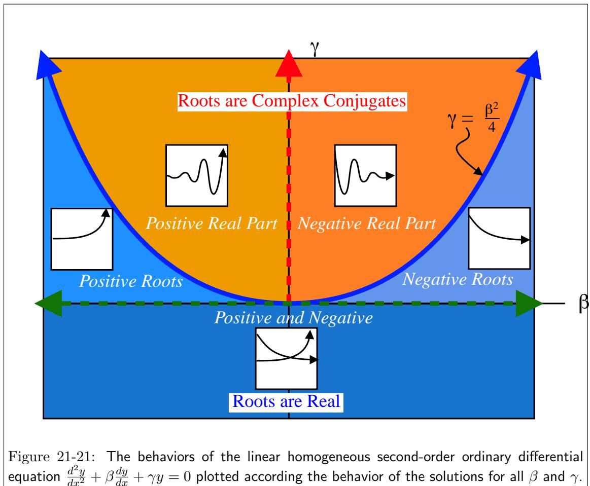
Figure 21-21: The behaviors of the linear homogeneous second-order ordinary differential equation  $\frac{d^2y}{dx^2} + \beta \frac{dy}{dx} + \gamma y = 0$  plotted according the behavior of the solutions for all  $\beta$  and  $\gamma$ .
