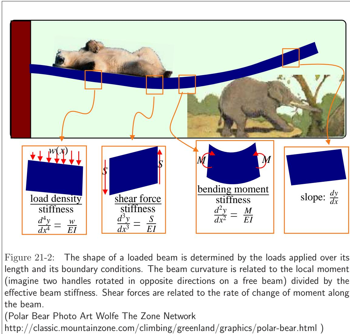
Figure 21-2: The shape of a loaded beam is determined by the loads applied over its length and its boundary conditions. The beam curvature is related to the local moment (imagine two handles rotated in opposite directions on a free beam) divided by the effective beam stiffness. Shear forces are related to the rate of change of moment along the beam.
