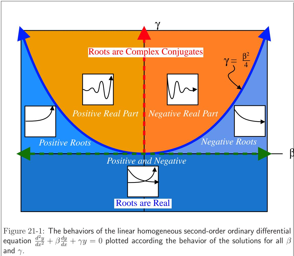
Figure 21-1: The behaviors of the linear homogeneous second-order ordinary differential equation  $\frac{d^2y}{dx^2} + \beta \frac{dy}{dx} + \gamma y = 0$  plotted according the behavior of the solutions for all  $\beta$  and  $\gamma$ .
