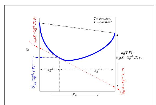
Figure 28-2: Illustration of how to determine the chemical potentials from a graph of  $\overline{G}(X_B)$  for a binary alloy.  $X_B^{arb}$  is an arbitrary composition where the tangent construction is performed.
