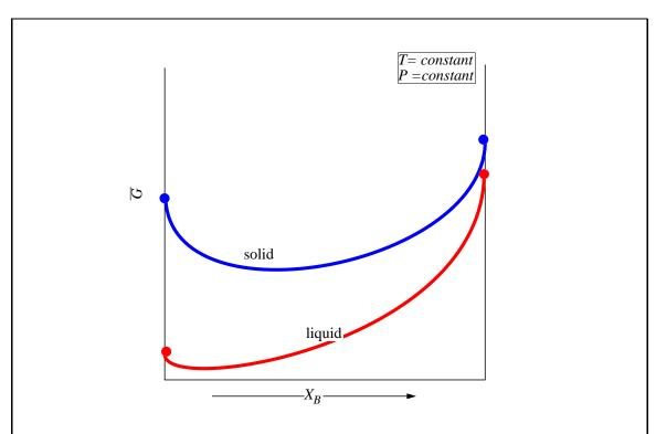
$Figure\ 28-3$ : Molar Gibbs Free Energies for a liquid and solid solution at a particular pressure and temperature.
