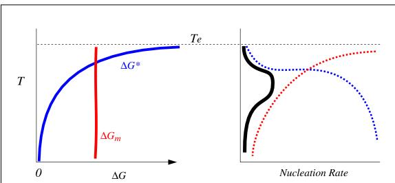
Figure 35-4: The competing effects of activated nucleation versus the rate of transfer to a nucleus.
