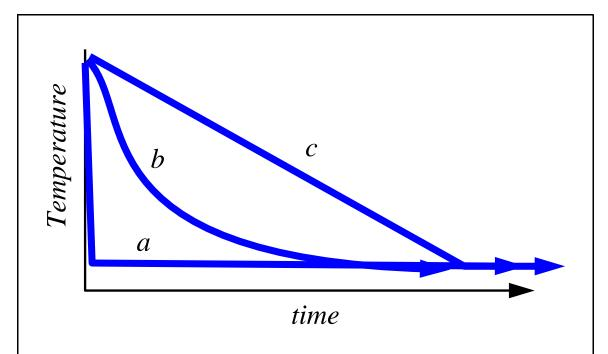
Figure 35-3: Three of a possible infinite number of cooling curves for one of the quenches illustrated in Fig. 35-2.
