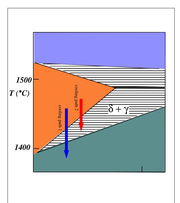
Figure 35-2: Example of two different processes that can initiate a phase transformation—however, the cooling path alone is insufficient to determine the type of microstructure that will result.
