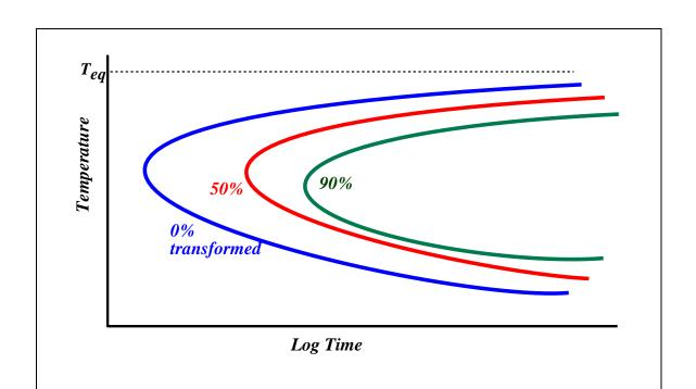
At temperatures just below the equilibrium transformation temperature, transformations take a long time since the nucleation rate is low. (Remember that at low driving forces, that heterogeneous nucleation is expected to dominate.) At large undercoolings, transformation times are limited by transport or by motion of atoms across the transformation interface.
