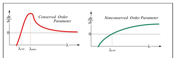
Figure 23-1: The amplification factor for spinodal decomposition and order-disorder reactions.
