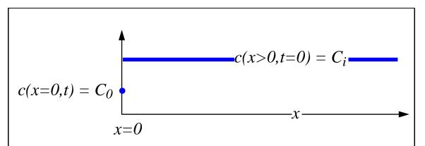
Figure 11-3: Semi-infinite, one-dimensional domain with BCs  $c(x=0,t)=C_0$  and  $J(x=\infty,t)=0$  and uniform initial conditions,  $c(x>0,t=0)=C_i$ .
