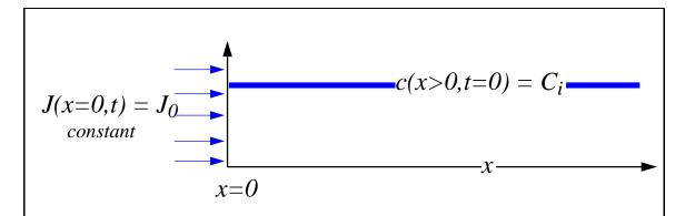
Figure 11-4: Semi-infinite, one-dimensional domain with BCs  $J(x=0,t)=J_0$  and  $J(x=\infty,t)=0$  and uniform initial conditions,  $c(x>0,t=0)=C_i$ . Because, material is constant flowing into the domain, the concentration at the boundary x=0 will be a function of time.
