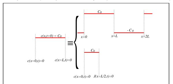
Figure 11-1: Illustration of equivalent initial and boundary conditions for a particular solution.
