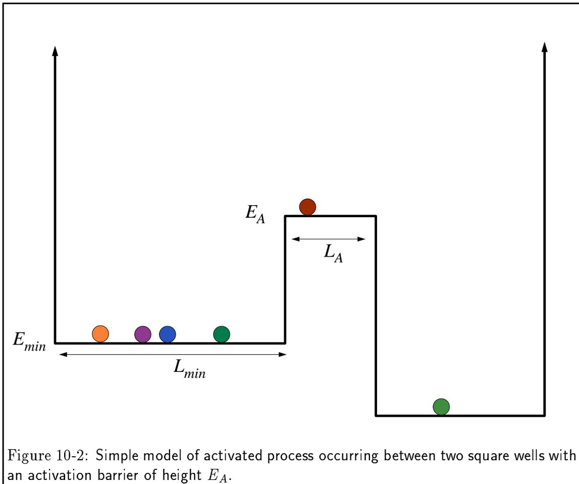
Figure 10-2: Simple model of activated process occurring between two square wells with an activation barrier of height  $E_A$ .
