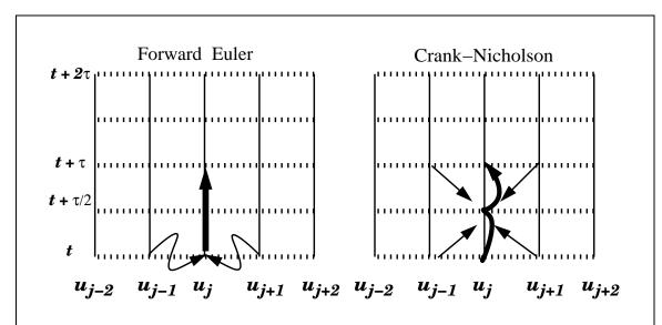
Figure 9-1: Illustration of the forward difference and implicit time-iteration methods. The implicit method uses values from the inferred solution to stabilize the numerical time-step.
