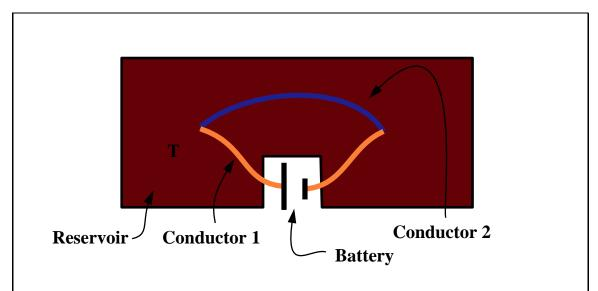
Figure 3-3: Experimental set-up for the Peltier effect. A perfect battery sets up a specified potential potential difference,  $\Delta\phi$ . As current,  $J_q$ , crosses the thermocouples, heat is produced and consumed depending on which material has a higher Fermi energy. Heat,  $J_Q$ , flows between the two junctions to maintain a constant temperature.
