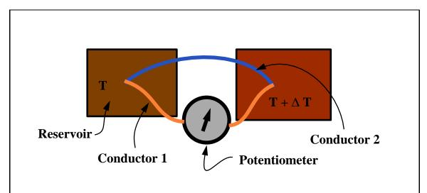
Figure 3-2: Experimental set-up for the Seebeck effect. A potentiometer measures the potential difference,  $\Delta \phi$ , between two conductor couples each at a different temperature.
